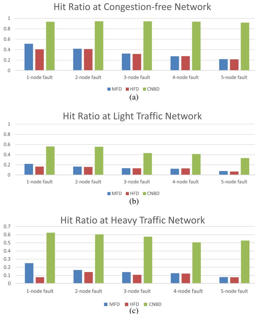
Fig. 6. Hit Ratio of MFD, HFD, and CNBD at (a) congestion-free network, (b) light traffic network, and (c) heavy traffic network.
