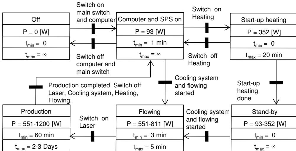
Figure 9: Petri-net of the laser sinter machine.
