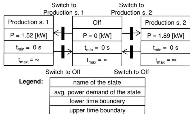
Figure 3: Petri-net of the grinding machine.
