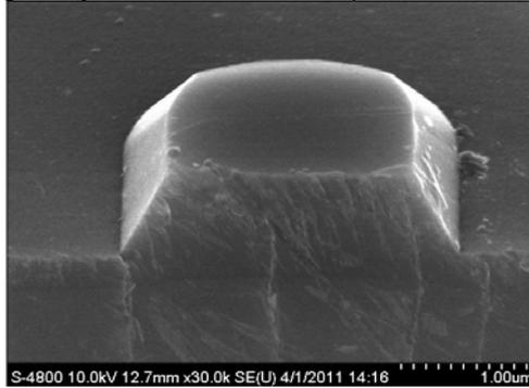
Fig 4. The etching results of <100> wafer
