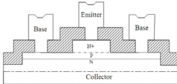
Fig 1. The profile of mesa SiGe HBT with Ploy silicon emitter
