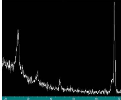
Fig 3. X-ray diffraction scan curves of epitaxial SiGe/Si wafer
