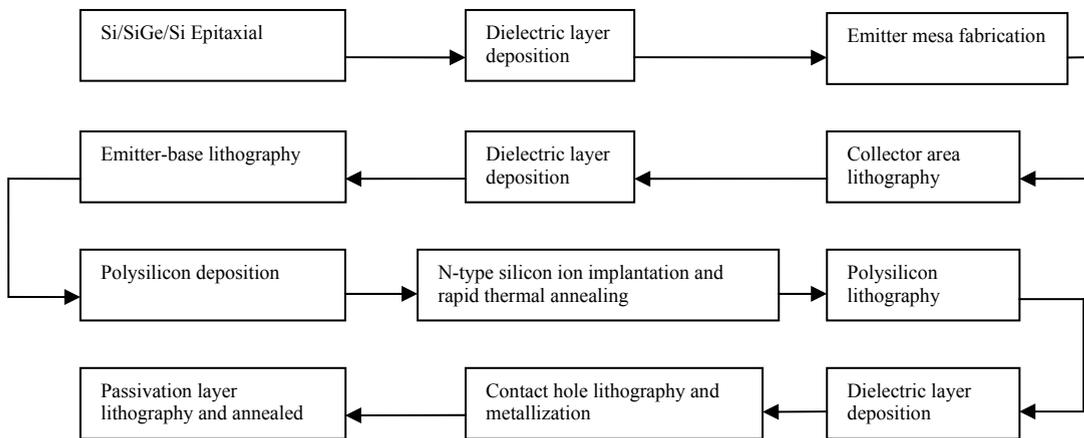
Fig 2. Process flow schematic diagram
